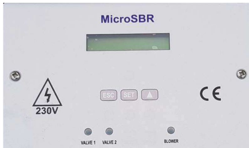
Figure 14: Controller of the OPTIMAX VIRO treatment plant
