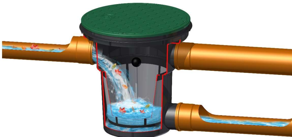
Figure 2: D400 AQ overflow rainwater filter - operation diagram
