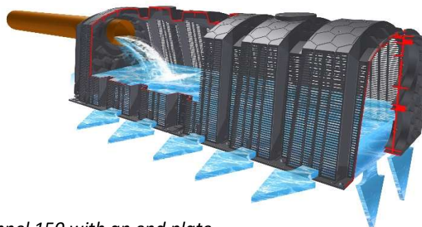
Figure 5: Infiltration tunnel 150 with an end plate
