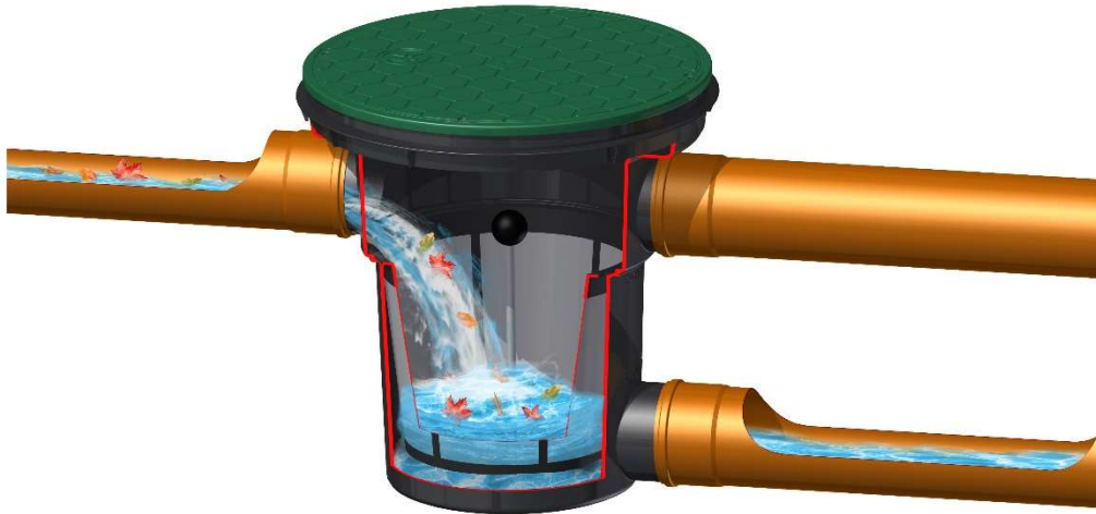
Figure 2: D400 AQ overflow rainwater filter - operation diagram
